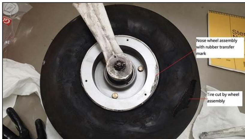
Figure 2 Damage on nose wheel assembly
