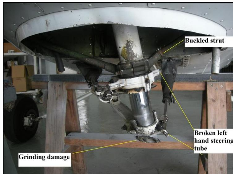
Figure 5 Damage of nose landing gear
