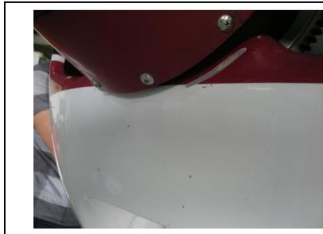
Figure 10 Rub mark on engine cowling
