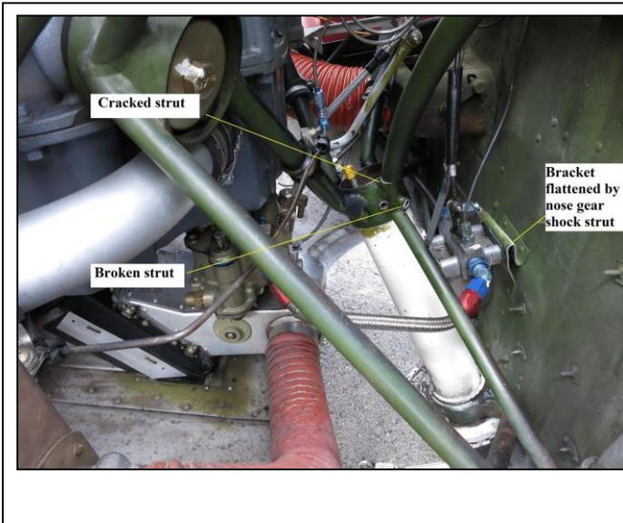
Figure 6a Damaged engine mount truss
