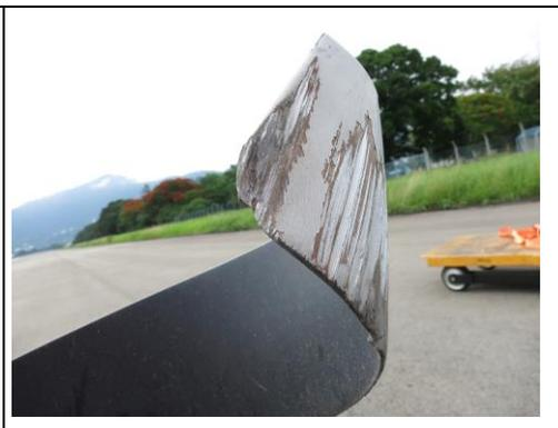
Figure 9 Damage of propeller blade
