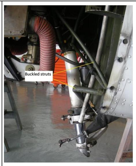
Figure 6b Buckled struts of truss
