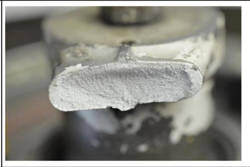
Figure 4 Broken nose gear fork at axle
