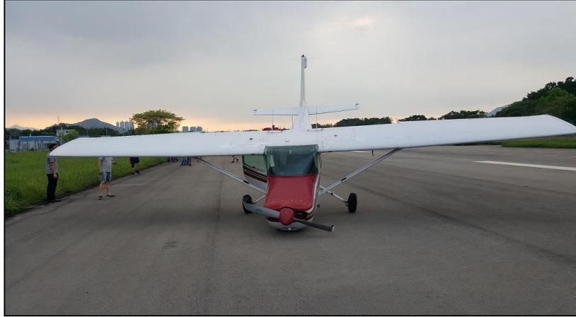
Figure 1 Aircraft stopped in a nose down position on Runway 11
