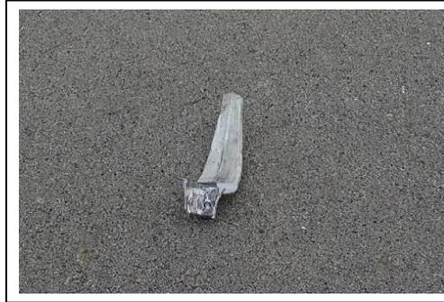
Figure 3 Broken nose wheel fork
