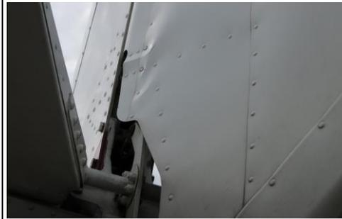
Figure 11 Wrinkled damage on the skin surface around the attachment point of rudder and rudder control cable
