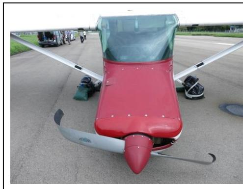
Figure 8 Propeller blades bent rearward
