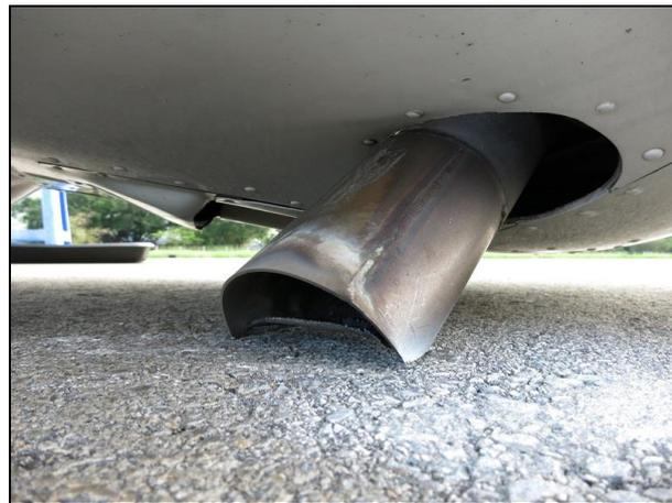
Figure 7 Grinding damage of exhaust pipe
