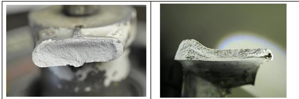
Figure 15 Broken nose gear fork at axle
