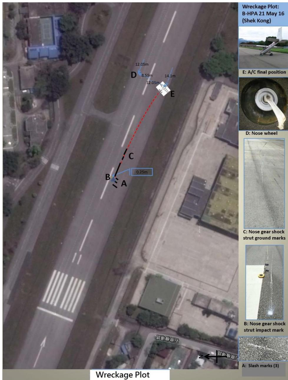
Figure 14 Wreckage Plot
